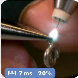
Its high heat conductivity makes working with this metal particularly problematic. This is why the welding spots tend to be smaller and not as deep.
