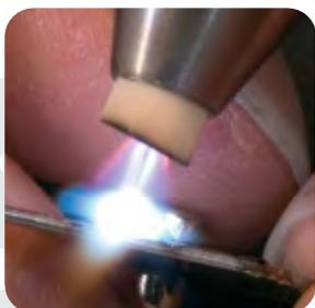
**9** You can use the same process to smooth the metal. This time use a little less power and put the electrode vertically next to the "mound of silver".
