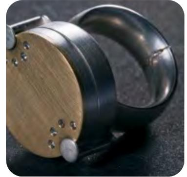
**2** When working with small or thin parts this effect is less pronounced, this is because the volume of metal is missing. A high metal volume would conduct the heat and direct it away from the working area too quickly. This is why the PUK produces very good results with loops or thin silver pieces.
